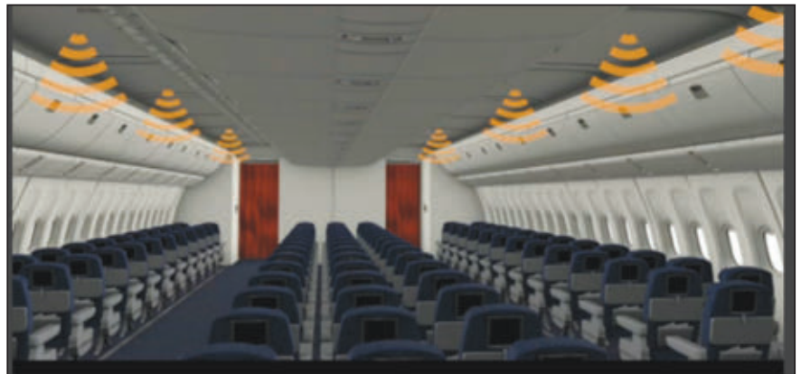
▲ Fig. 12 The leaky feeder antennas are mounted in the aircraft ceiling above the aisles.
